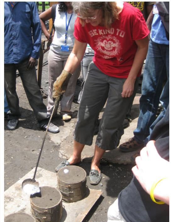
*Pouring molten metal into the molds.*
