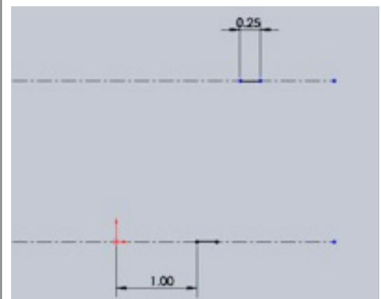
Connect the lines on each side and **Smart Dimension** one by clicking on the angled line and then the centerline to make the angle 85 degrees.
