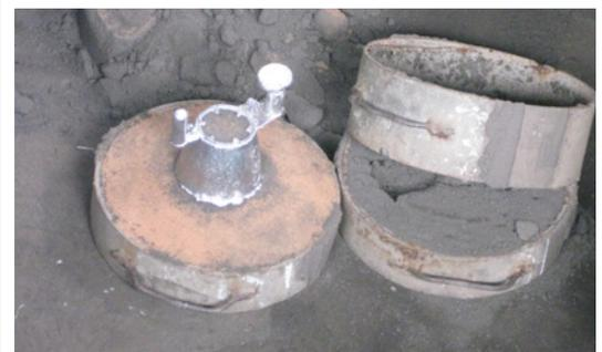
*A cast corn sheller with sprues attached.*
