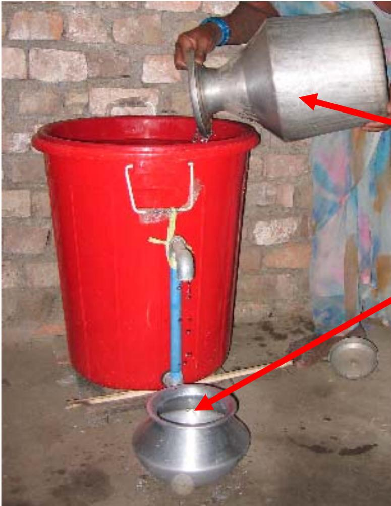
1. Pour water into top basin. Water will pass through filter and flow up the pipe
