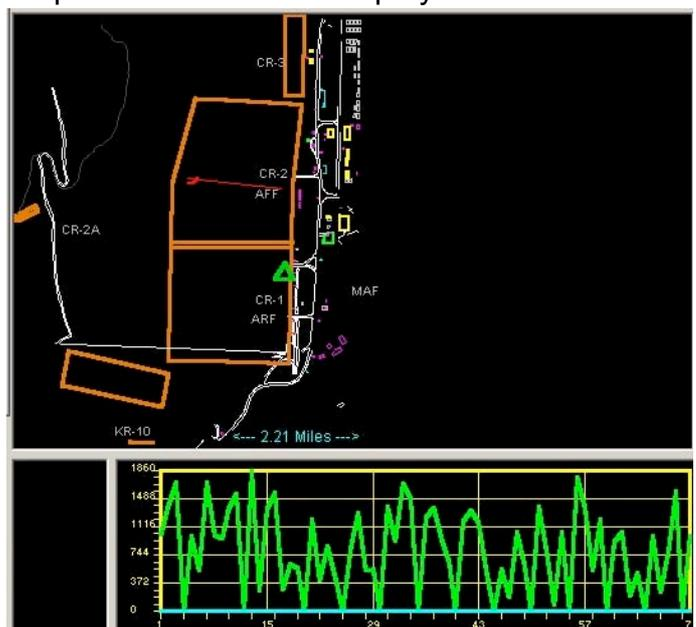
large open areas is provided by a centimeter-level accuracy Z-surveyor. This utilizes a base station at a known surveyed position and connected via radio link to the roving survey vehicle. Position information is passed from the GPS receiver to the computer using a NMEA standard GPGGA serial message. The laptop computer receives serial messages from the towed sensors through PCMCIA interfaces.
