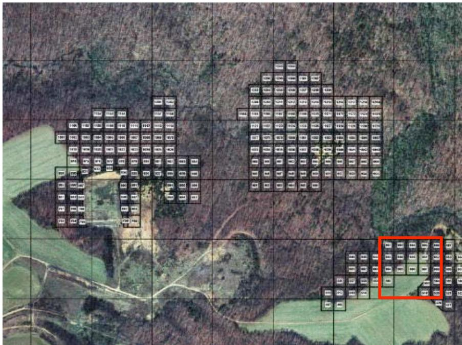
The Overview can be broken down into larger grids, which would be highlighted when the REST filters indicate a presence of explosives. The individual 50x50 or 100x100 sub-grids can then be identified through the higher resolution settings. Anything obviously noticeable would also be entered on the map, so a living system is developed
