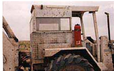
Fig. 3: Polycarbonate Windows on a Armoured Backhoe Cab
