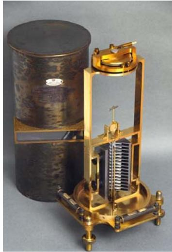
Figure 5.2.1: Example of electrostatic voltmeter.
