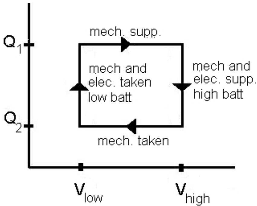
Figure 10-5: Charging Cycle energy movement
