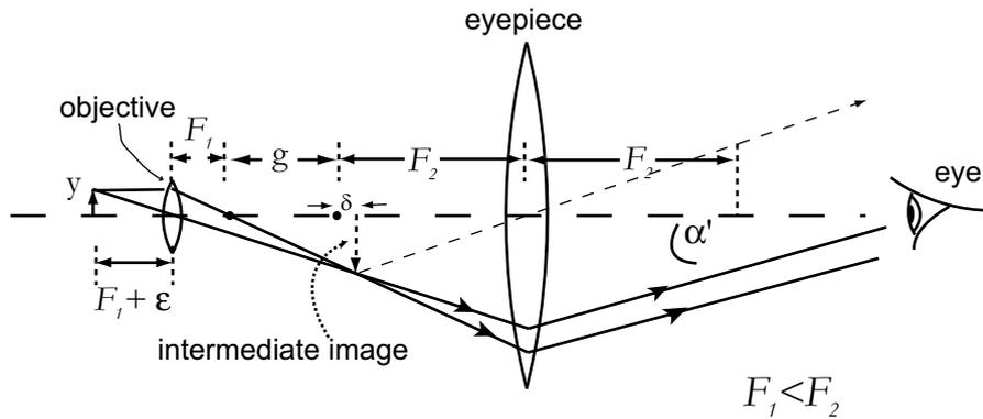
Figure 1: Ray diagram for a microscope
