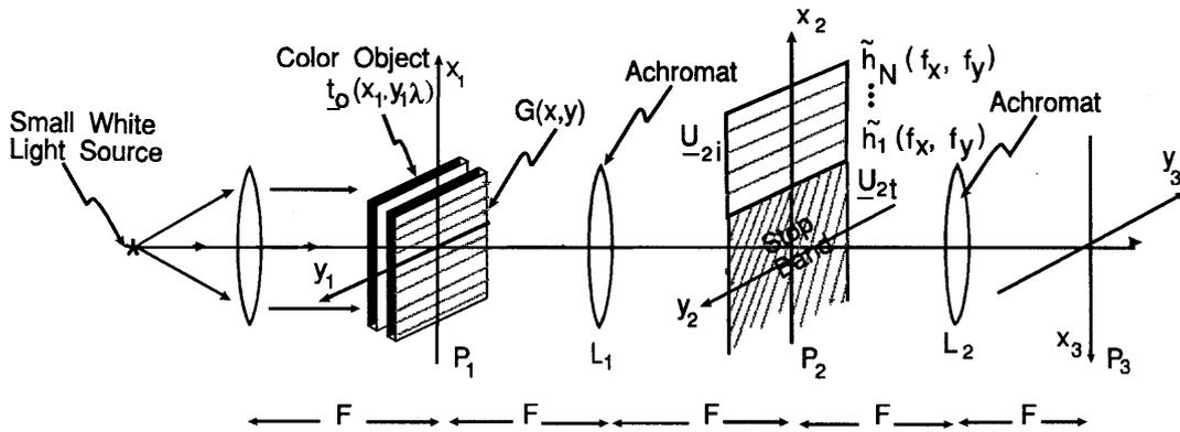
Figure 1: Typical white light optical processing system for a color object
