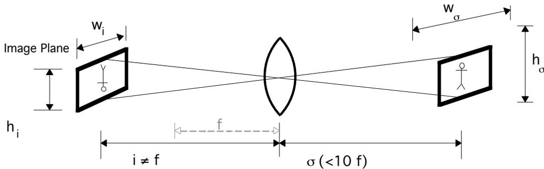
$$\text{magnification } m = \frac{h_i}{h_\sigma} = \frac{w_i}{w_\sigma} = i/\sigma \quad \text{And, } \frac{1}{f} = \frac{1}{i} + \frac{1}{\sigma}$$
