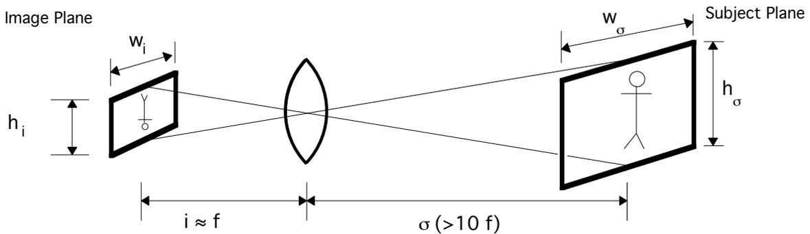
$$\text{magnification } m = \frac{h_i}{h_\sigma} = \frac{w_i}{w_\sigma} = i/\sigma \approx f/\sigma \text{ (if } \sigma > 10 f \text{)}$$
