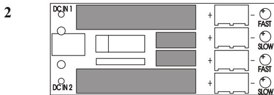
Next, solder in the four large power resistors. R1 and R2 are the larger resistors with square cross sections; R3 and R4 have circular cross sections. The large resistors are for fast charging, and the small ones are used for slow charging. You can mount them in any orientation, but you should try to make the markings on the resistors visible.
