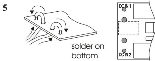
Finally, connect the power supply leads to the PCB. Pass the insulated wires through the larger, inner holes from the bottom of the board, then bend them out and solder them to the outer holes. The larger holes and the wire insulation provide a strain relief that should prevent your wires from breaking off with use. Either wire can go to either hole. J1, a DC input jack, is not used this year.
