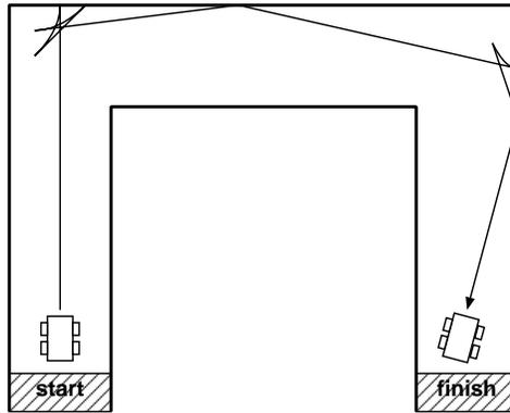
Figure 7.4: A robot using feedback to navigate
