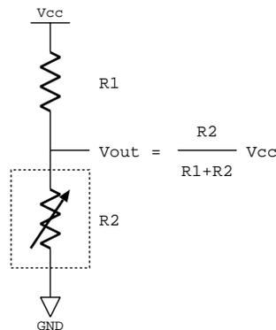
Figure 5.3: Resistive Analog Sensor Circuit
