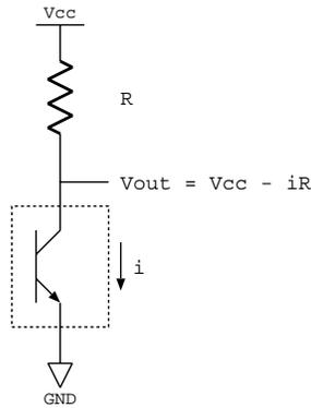
Figure 5.5: Transistive Analog Sensor Circuit
