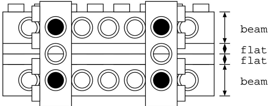
Figure 6.2: A Simple Braced Structure
