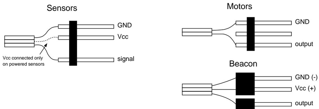
Figure 4.7: 6.270 connector standard
