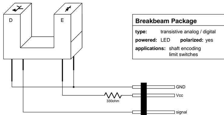
Figure 5.7: Breakbeam sensor package
