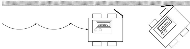
Figure 7.6: Wall following and a jammed robot
