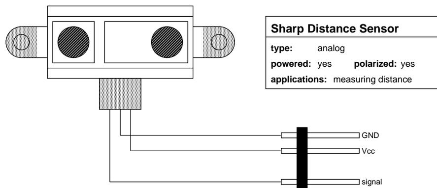
Figure 5.8: Sharp Distance Sensor
