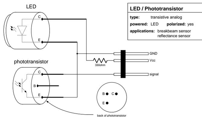
Figure 5.6: LED and Phototransistor
