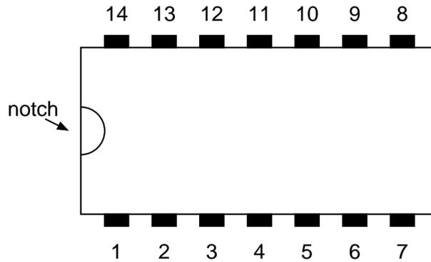
Figure 4.6: Top view of a 14-pin DIP
