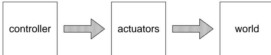
Figure 7.1: Open loop information flow
