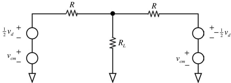
And “half-circuit” analysis is nothing more than an expression of superposition. For the common-mode half-circuit, we set  $v_2$  to zero and calculate responses. For the differential half-circuit, we set  $v_{cm}$  to zero.
