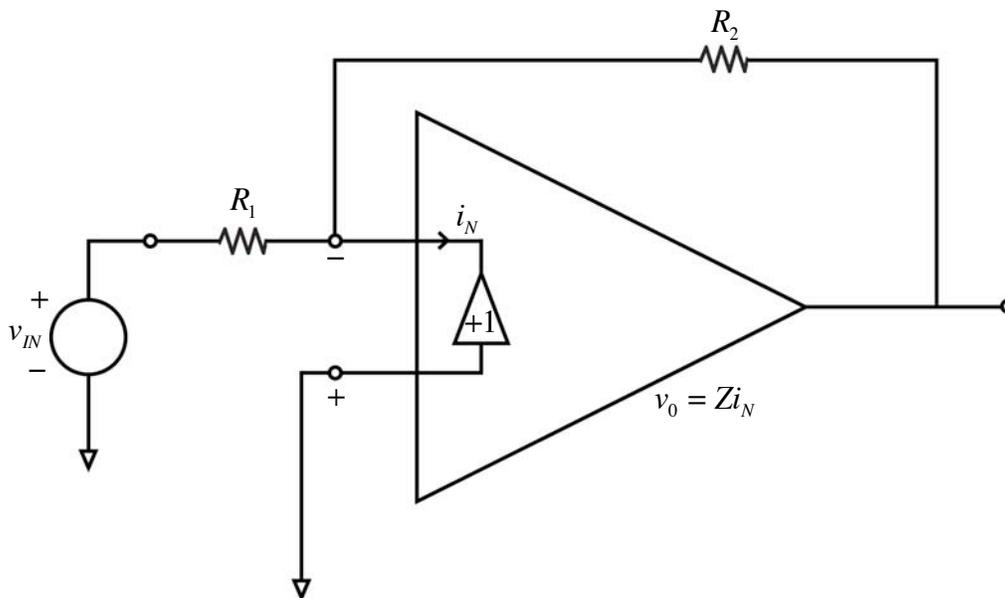
A start to the analysis is to observe that, as in the case of the voltage op-amp,  $V_+ = V_- (= 0)$ . The reasons are different, of course. For the voltage op-amp, it was negative feedback, combined with infinite gain, that forced  $V_+ = V_-$ . Here,  $V_+ = V_-$  by construction, because we have placed a voltage buffer between them.
