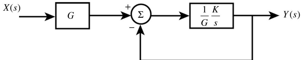
Here,  $G$  is the ideal gain, and the dynamics of the op-amps are captured by  $\frac{k}{s}$ . Show that as the gain  $G$  is varied, this system exhibits a constant gain-bandwidth product.
