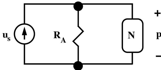
Figure 4: An acoustic circuit consisting of a volume velocity source, an acoustic resistance, and an unknown element  $N$  (acoustic mass or acoustic compliance).
