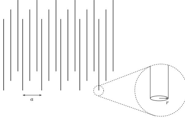
**Figure 2:** Array of rods confining the electrons in space.
