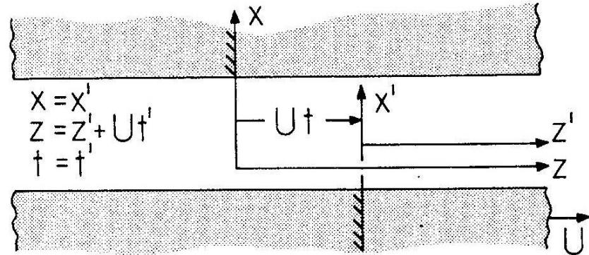
Rotor and stator reference frames  $z'$  and  $z$ .
