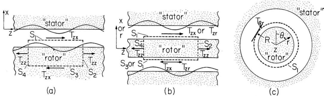
Typical "air-gap" configurations in which a force or torque on a rigid "rotor" results from spatially periodic sources interacting with spatially periodic excitations on a rigid "stator." Because of the periodicity, the force or torque can be represented in terms of the electric or magnetic stress acting at the air-gap surfaces  $S_1$ : (a) planar geometry or developed model; (b) planar or cylindrical beam; (c) cylindrical rotor.
