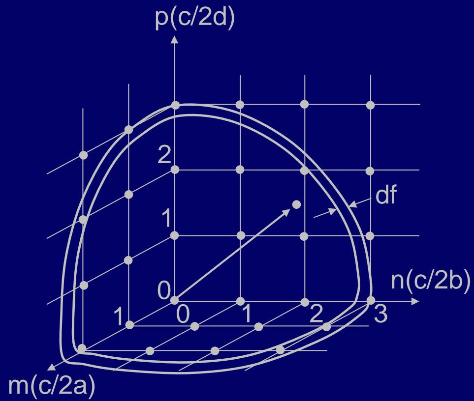
$$f_{m,n,p} = \sqrt{\left(\frac{cm}{2a}\right)^2 + \left(\frac{cn}{2b}\right)^2 + \left(\frac{cp}{2d}\right)^2}$$
