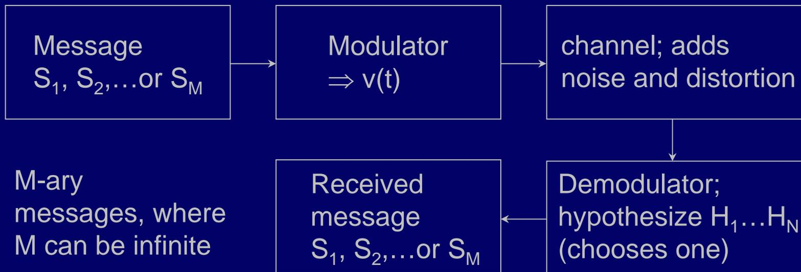
The channel can be radio, optical, acoustic, a memory device (recorder), or other objects of interest as in radar, sonar, lidar, or other scientific observations.
