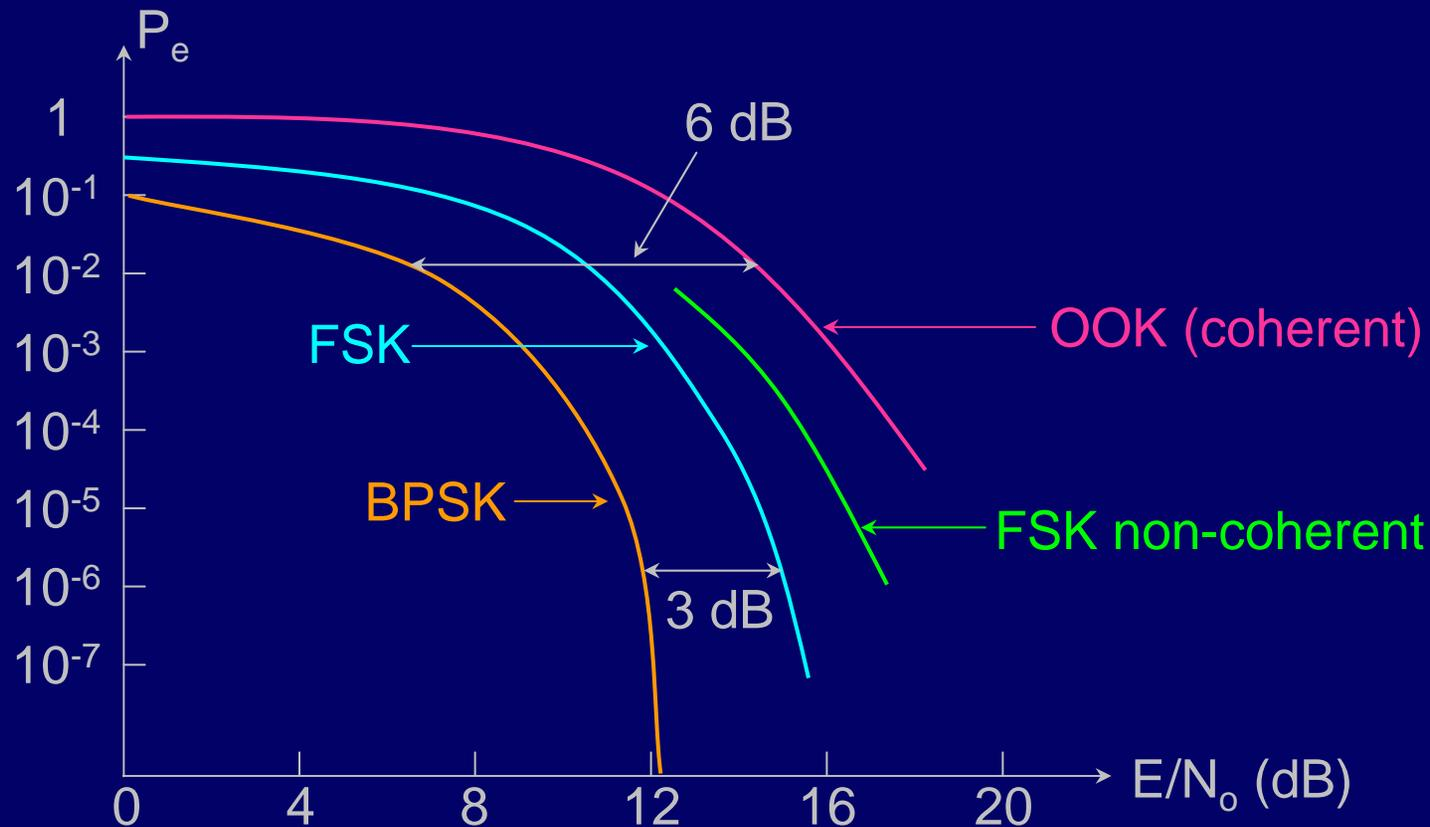
**Non-coherent FSK:** carrier is unsynchronized so that both sine and cosine terms admitted, increasing noise. Such “envelope detectors have a different form of  $P_e(E/N_0)$ .”
