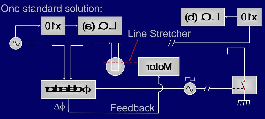
"Line stretcher" varies path so that  $\Delta \phi \cong 0$ Communications and telemetry systems can similarly be phase synchronized
