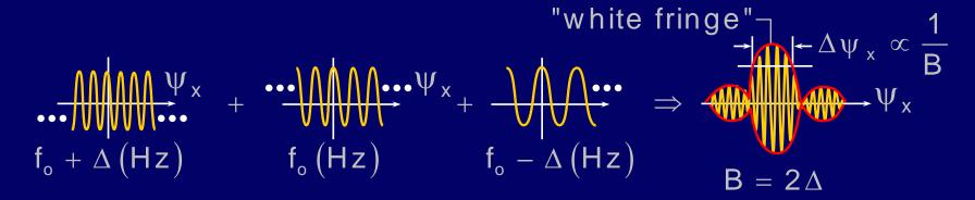
A delay line in one interferometer arm can redirect the strong white fringe in other directions.
