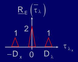
Example: 2 small duplicate antennas separated by  $D_{\lambda}$  in the x direction
