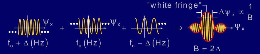
A delay line in one interferometer arm can redirect the strong white fringe in other directions.
