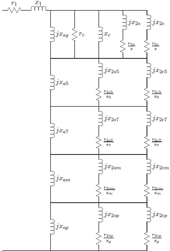
Figure 21: Extended Equivalent Circuit
