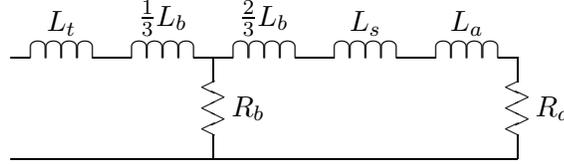
Figure 11: Equivalent Circuit: Double Bar
