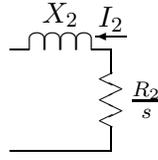
Figure 4: Rotor Equivalent Circuit
