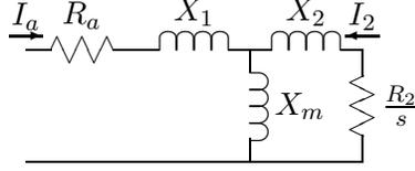
Figure 2: Equivalent Circuit
