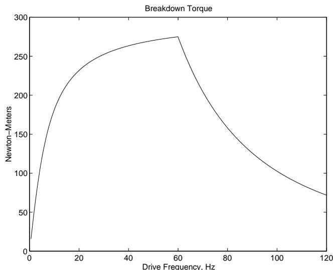
Figure 18: Torque-Capability Curve For An Induction Motor
