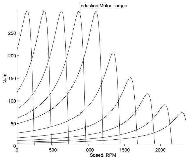
Figure 17: Idealized Torque-Speed Curves: Zero Stator Resistance
