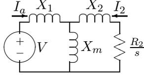
Figure 15: Idealized Circuit: Ignore Armature Resistance
