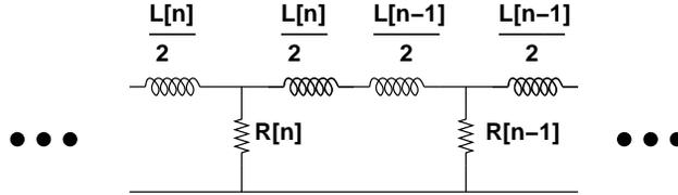
Figure 9: Slot Impedance Ladder Network
