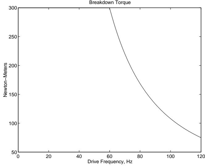
Figure 19: Idealized Torque Capability Curve: Zero Stator Resistance
