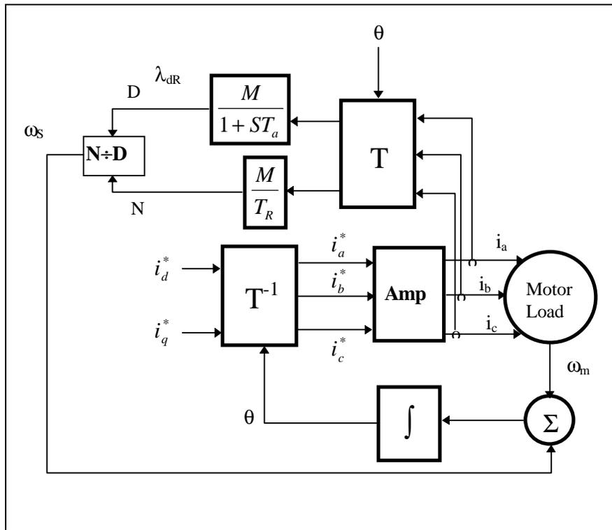
Figure 20: Field Oriented Controller
