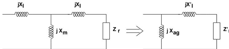
Figure 5: Effect of Skew on Equivalent Circuit
