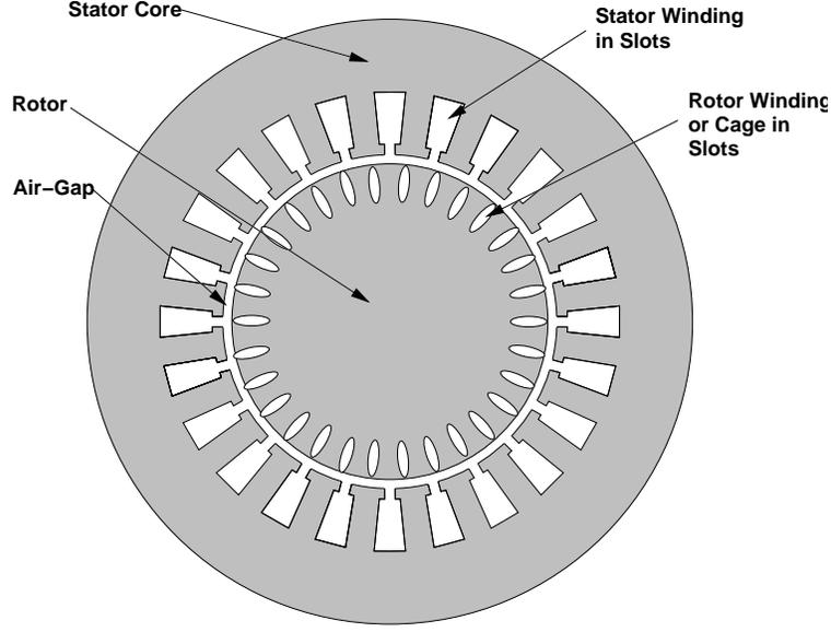
Figure 1: Axial View of an Induction Machine
