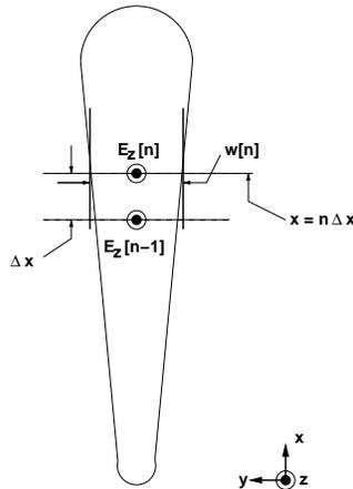
Figure 8: Slot Geometry Notation
