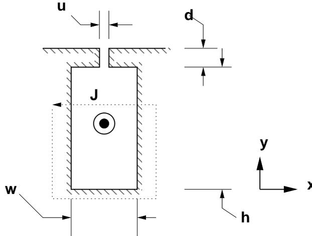
Figure 6: Stator Slot Geometry for Leakage Calculation
