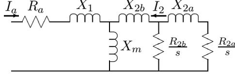
Figure 12: Equivalent Circuit: Double Cage Rotor
