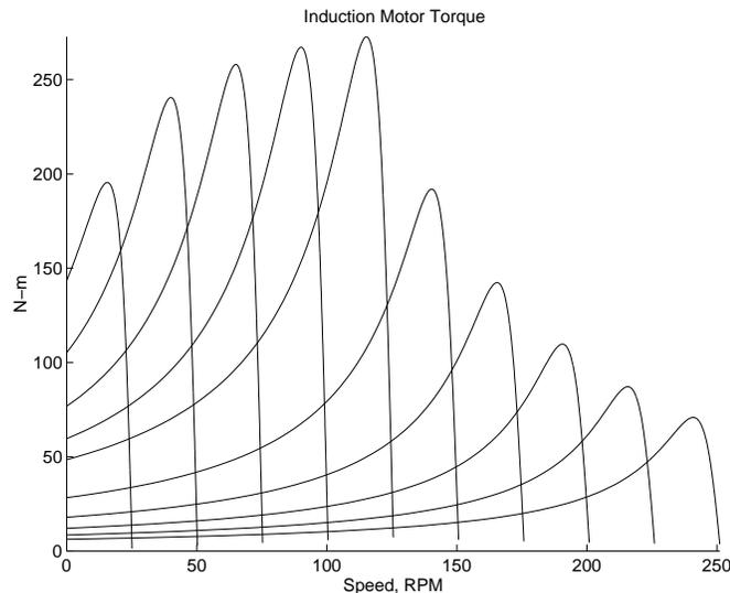
Figure 14: Induction Machine Torque-Speed Curves
