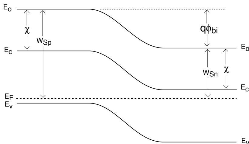
$$\begin{aligned} q\phi_{bi} &= W_{Sp} - W_{Sn} = (E_C - E_F)|_{x \ll 0} - (E_C - E_F)|_{x \gg 0} \\ &= kT \ln \frac{n_o(x \gg 0)}{n_o(x \ll 0)} \end{aligned}$$
