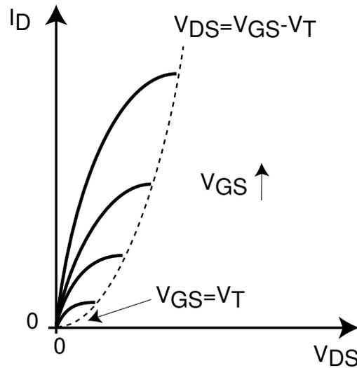
$$I_D = \frac{W}{L} \mu_e C_{ox} (V_{GS} - V_T - \frac{1}{2} V_{DS}) V_{DS}$$
