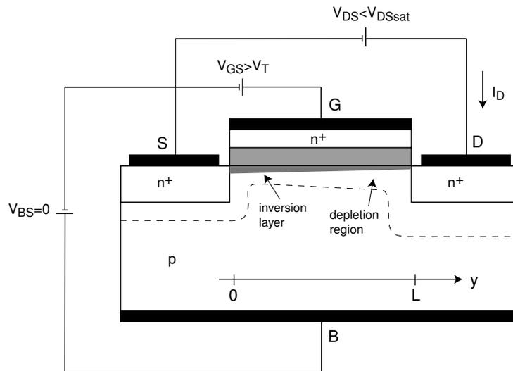
Inversion layer everywhere under gate. Lateral field set up along channel  $\rightarrow$  current flows.
