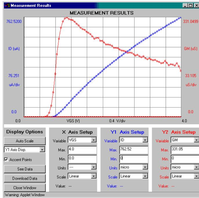
$g_m$  in linear regime ( $V_{DS} = 0.1 \text{ V}$ ) for  $L_g = 0.18 \mu\text{m}$  MOSFET:
