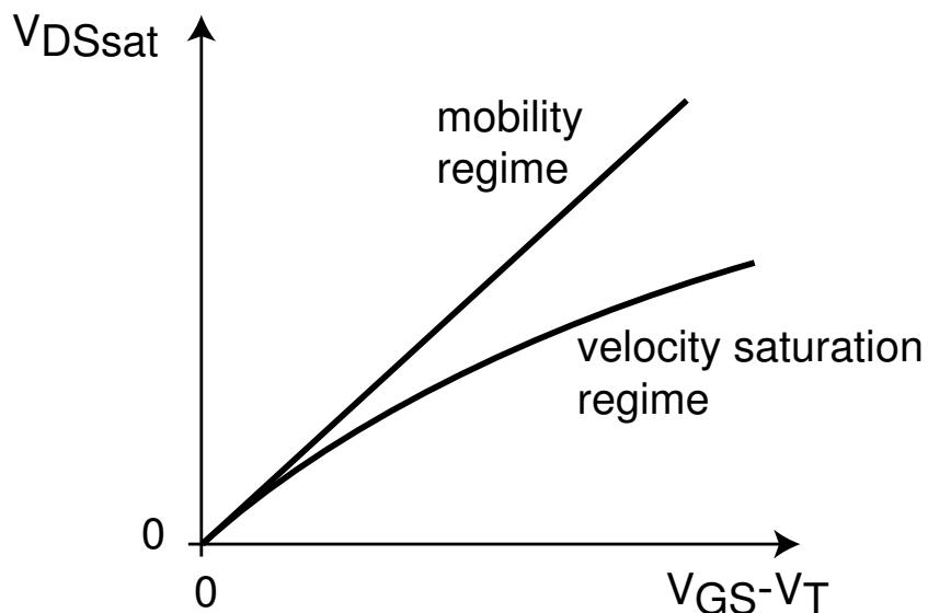
Velocity saturation results in *premature current saturation* and less current:
