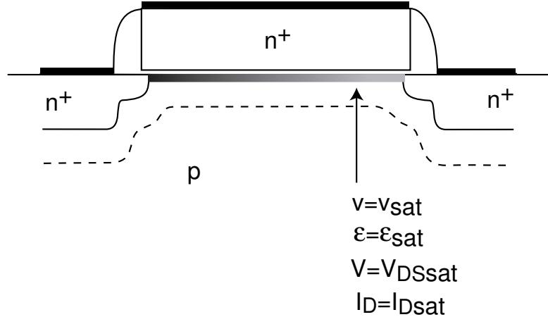
Bottleneck is current flowing through  $v_{sat}$  region:
