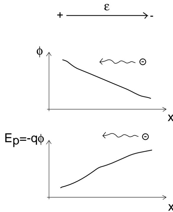
Electron trades potential energy by kinetic energy as it moves to the left  $\rightarrow$  *total electron energy unchanged*
