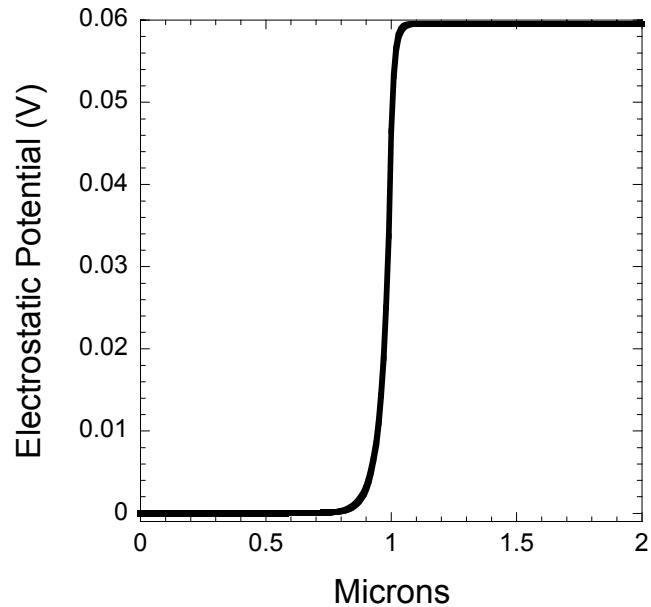
In equilibrium, the carrier concentration is balanced by an internal electrostatic potential...
