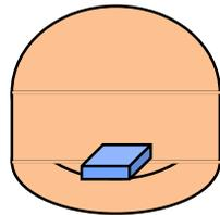
If the device is fabricated with a substrate that is transparent to the emitted radiation, then light can be extracted from the 4 sides and bottom of the device as well as from the top. This increases the extraction efficiency by a factor of 6!
