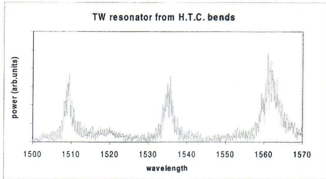
**Q of resonance indicates 0.3 dB loss per corner**
