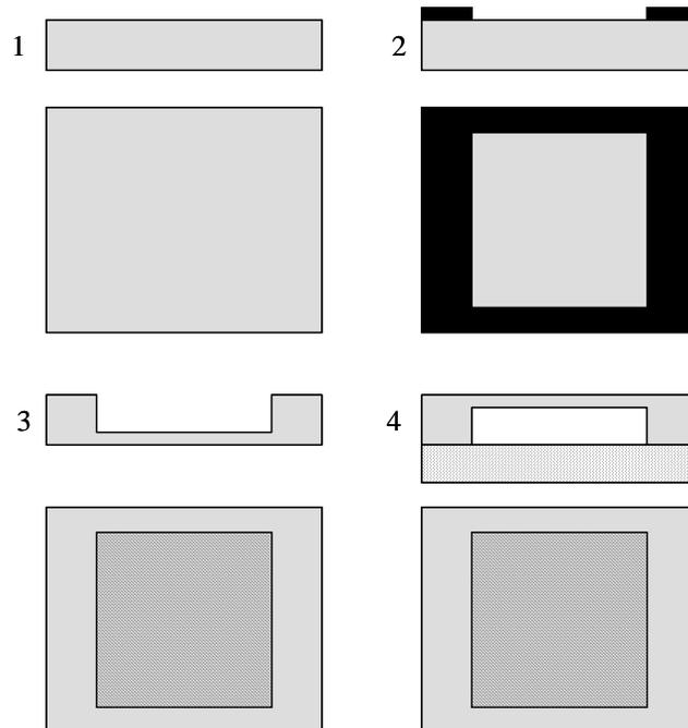
Figure 1: Process flow for a pressure-sensing silicon diaphragm.
