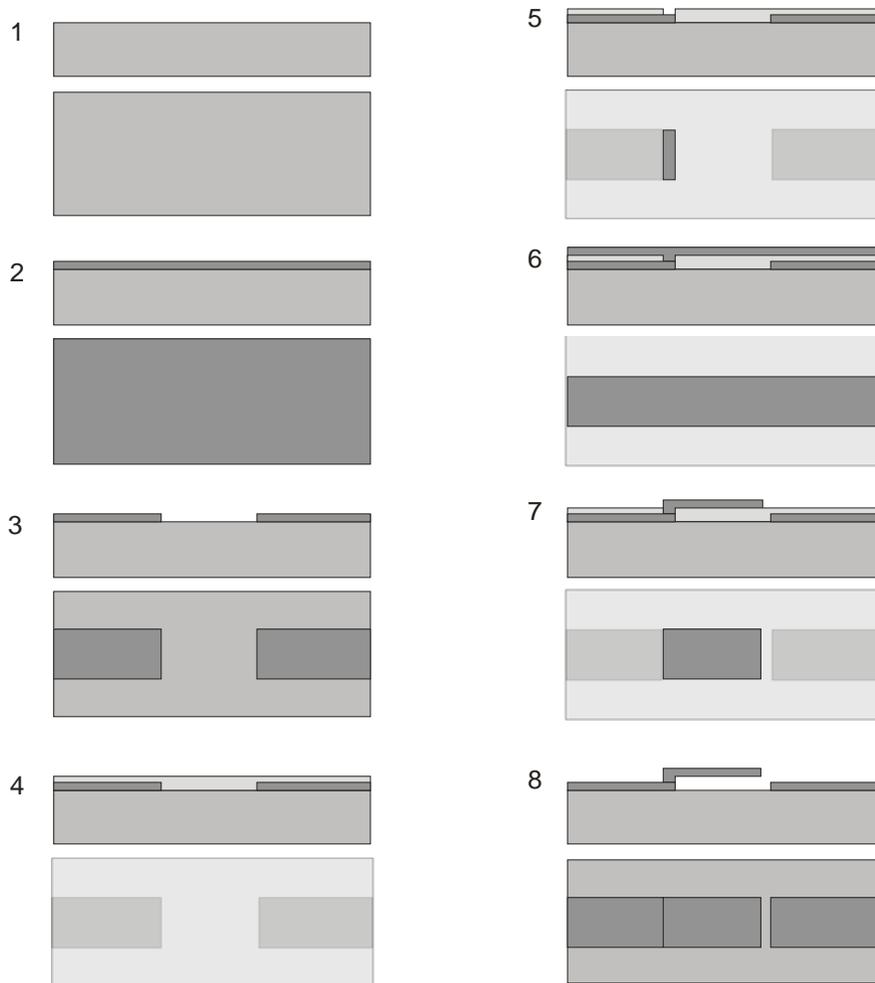
Figure 1. Process flow for a surface-micromachined cantilever.
