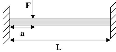
$$\begin{aligned} EI \frac{d^3 w}{dx^3} &= -F \langle x - a \rangle^0 + C_1 \\ EI \frac{d^2 w}{dx^2} &= -F \langle x - a \rangle^1 + C_1 x + C_2 \\ EI \frac{dw}{dx} &= -\frac{F}{2} \langle x - a \rangle^2 + \frac{1}{2} C_1 x^2 + C_2 x + C_3 \\ EI w &= -\frac{F}{6} \langle x - a \rangle^3 + \frac{1}{6} C_1 x^3 + \frac{1}{2} C_2 x^2 + C_3 x + C_4 \end{aligned}$$
