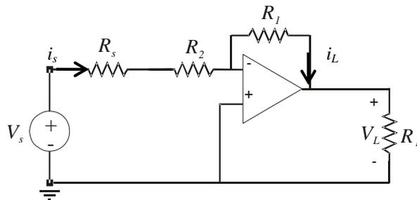
c) The gain G is defined as the ratio of the output voltage to the input voltage, or  $V_L / V_s$ .
