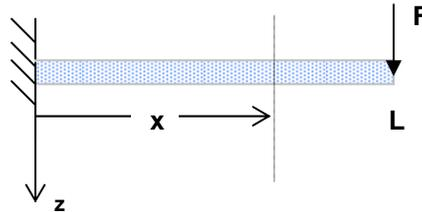
the differential equation of beam bending is:
