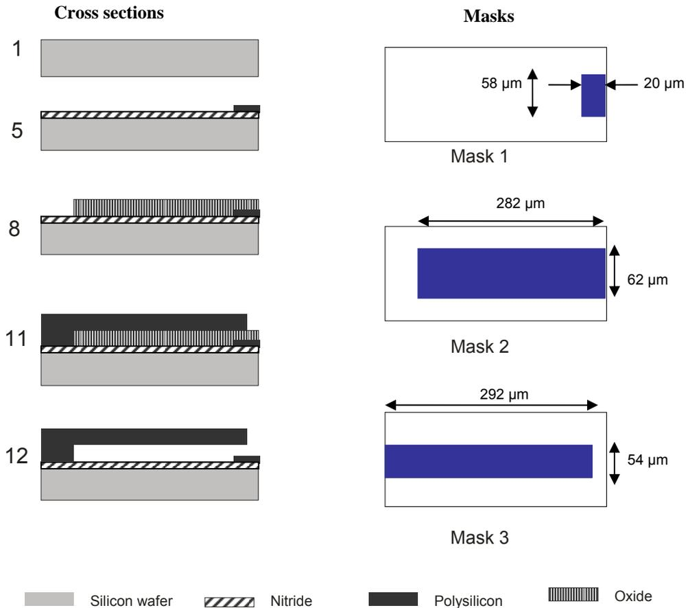
Figure 1. Process flow and mask set for micromachined cantilever switch
