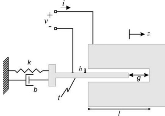
The gap  $g$  between the finger tip and the electrode can be expressed in terms of the displacement  $z$  as follow,
