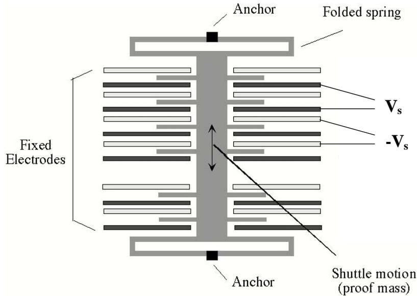
The circuit assumed here is vastly simplified; we will learn more about accelerometer readouts in the case studies. In the meantime, we assume that voltages are applied to the fingers in pulses with an amplitude  $V_s = 2.5$  V. We will look at the noise from various sources *while the pulse is applied* (in other words, we don't look very long, so it looks like DC.) However, we will assume a finite bandwidth due to the remainder of the circuit, which is not shown here.
