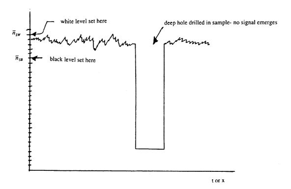
Note that at one point on the sample a hole is drilled so that we can determine the true background level. That is, no signal can emerge from the hole. The level  $\overline{n_{sw}}$  corresponds to a current at the noise bottleneck that is only 2% of the input beam current.
