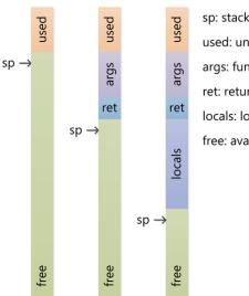
sp: stack pointer (data) used: unavailable stack args: function arguments ret: return address (code) locals: local variables free: available stack
