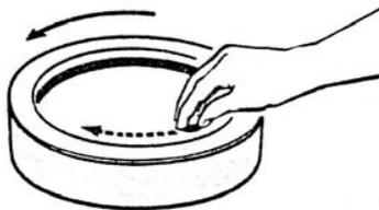
The direction of rotation of the sample during polishing
