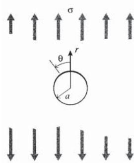
Figure 2: Circular hole in a uniaxially stressed plate
