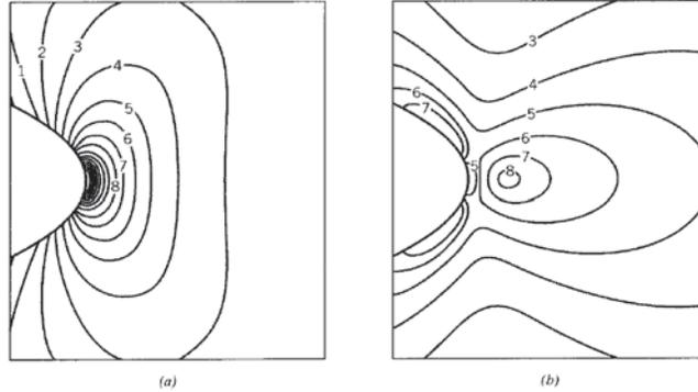
Figure 5: Stress field in the vicinity of an elliptical hole, with uniaxial stress applied in  $y$ -direction. (a) Contours of  $\sigma_y$ , (b) Contours of  $\sigma_x$ .
