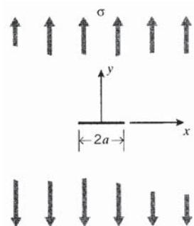
Figure 6: Sharp crack in an infinite sheet.
