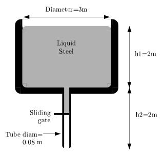
In a university laboratory, experimentation on this scale is completely unpractical, so researchers build a  $\frac{1}{100}$  scale miniature ladle to test new technologies. Their model ladle has a liquid steel height of 2 cm and diameter of 3 cm, the tube draining it is 2 cm long and 0.8 mm in diameter, etc.
