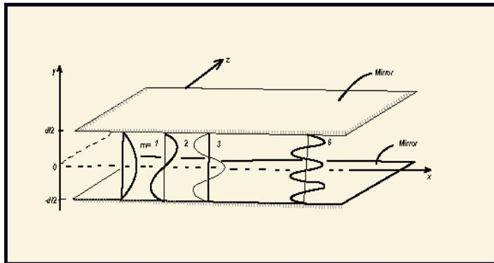
Field distributions of the modes of a planar-mirror waveguide
