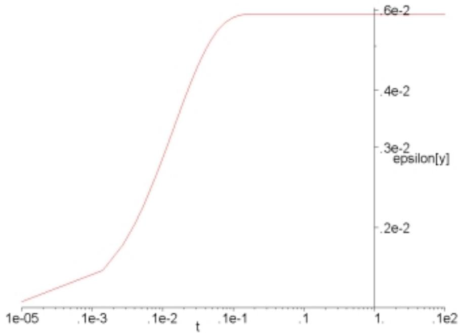
We might expect the  $(1-2*\nu)$  factor to drive the strain to zero as  $\nu$  approaches 0.5, but the tensile modulus is also dropping substantially, and the strain is observed to rise. The material does not become fully rubbery, and maintains a finite compressibility.
