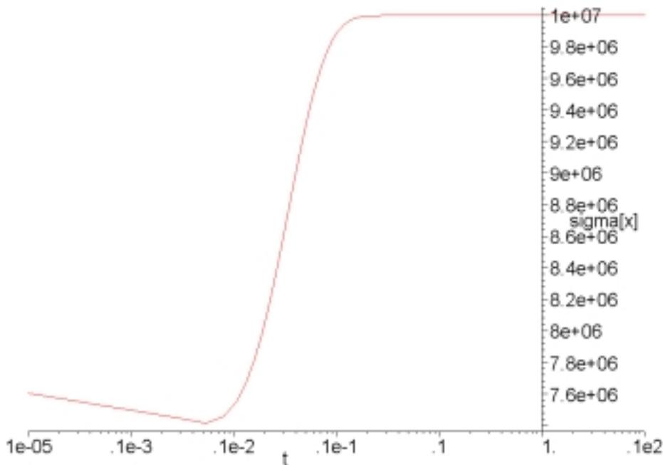
Note that the transverse stress becomes equal to the vertical stress (i.e. the stress state becomes hydrostatic) as the relaxation completes and the material approaches a rubbery state.
