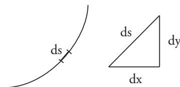
Figure 1: Straight line approximation of arc length.
