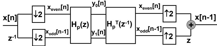
$$H_p(z) = \begin{bmatrix} H_{0,\text{even}}(z) & H_{0,\text{odd}}(z) \\ H_{1,\text{even}}(z) & H_{1,\text{odd}}(z) \end{bmatrix} \longrightarrow \text{Polyphase Matrix}$$
