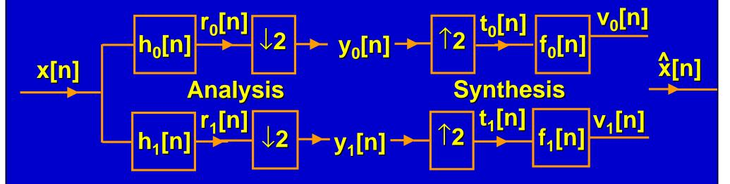
$$h_1[n] = \begin{array}{c} \frac{1}{\sqrt{2}} \\ 0 & 1 \\ \hline \\ \frac{-1}{\sqrt{2}} \end{array} \qquad f_1[n] = \begin{array}{c} \frac{1}{\sqrt{2}} \\ \hline \\ -\frac{1}{\sqrt{2}} \end{array}$$
