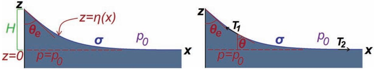
Figure 6.1: Calculating the shape and maximal rise height of a static meniscus.
