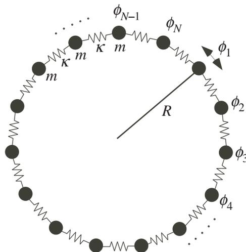
Figure 2:  $N$  identical masses  $m$  arranged on a circle, connected with spring constants  $\kappa$ , and allowed to slide freely on the circle, where  $\phi_\ell$  denotes the angular displacement of the  $\ell$ -th mass from its initial position (equally spaced).
