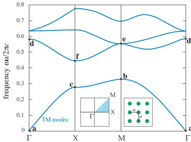
Figure 3: TM band diagram of a square lattice (lattice constant  $a$ ) of circular dielectric rods (right inset) plotted around the boundary of the irreducible Brillouin zone (left inset). Various points (black dots) are labelled with letters (a–f) for future reference.
