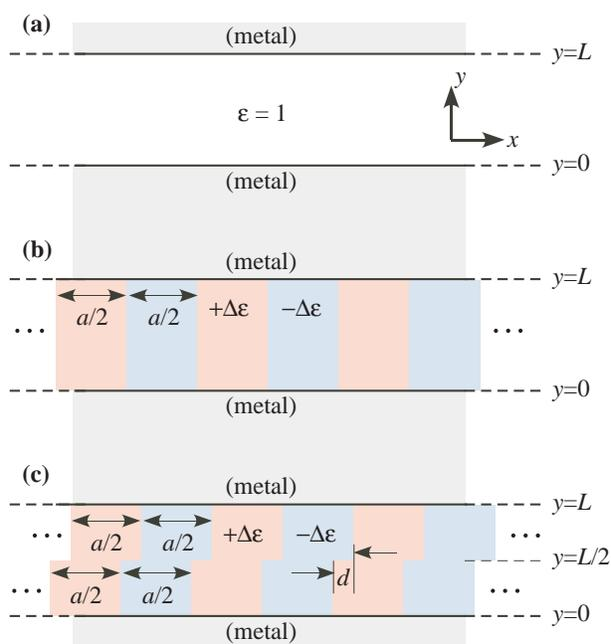
Figure 1: (a) Schematic of a 2d metal waveguide of width  $L$ , which supports modes propagating along the  $x$  direction. (b) A perturbation  $\pm\Delta\varepsilon$  is introduced via two periodic layers of thickness  $a/2$  filling the waveguide. (c) The perturbation is modified: for half of the thickness ( $y \in [0, L/2]$ ), the layers are shifted in the  $x$  direction by a distance  $d$ .
