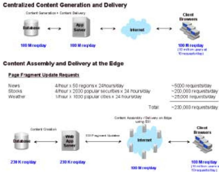
**Figure 1.10.** Comparison of traditional server access versus edge assembly.
