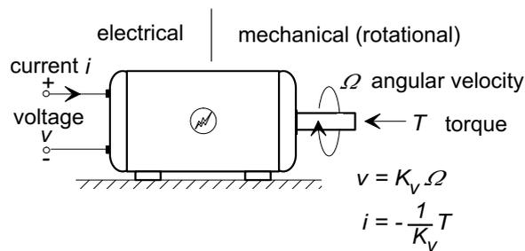
A transducer is bi-directional, that is it can transmit power  $P$  in both directions, so that the motor can also act as a generator.
