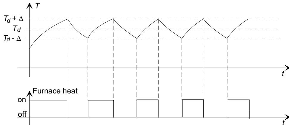
Notice that the temperature rises while the furnace is on, and falls while it is off. The thermostat acts to keep the temperature centered about the desired value  $T_d$  (known as the *set-point*).
