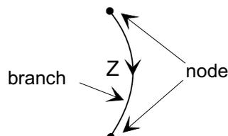
The impedance is drawn as a graph *branch* between two *nodes*. Nodes represent junctions between the elements in the circuit. The arrow on the branch indicates both the assumed direction of voltage drop across the element, and the assumed current direction.
