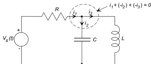
We will define a junction as a *node*, and if there are  $n$  circuit branches attached to a node
