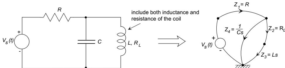
$$\begin{aligned} Z &= Z_1 + Z_4 \parallel (Z_2 + Z_3) \\ &= Z_1 + \frac{Z_4(Z_2 + Z_3)}{Z_4 + Z_2 + Z_3} \\ &= R + \frac{(1/sC)(R_L + Ls)}{1/sC + R_L + Ls} \\ &= R + \frac{R_L + Ls}{LCs^2 + R_LCs + 1} \end{aligned}$$
