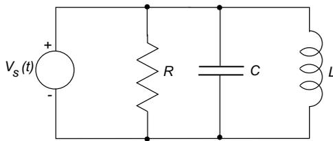
$$\begin{aligned} \frac{1}{Z} &= \frac{1}{1/sC} + \frac{1}{sL} + \frac{1}{R} \\ &= sC + \frac{1}{sL} + \frac{1}{R} \\ &= \frac{LCRs^2 + Ls + R}{RLs} \end{aligned}$$
