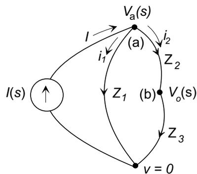
Let  $Z_1 = 1/sC$ ,  $Z_2 = R$ , and  $Z_3 = sL$ . We will use  $V_o(s) = I_2(s)Z_3$  (at node (b)), and find  $I_2(s)$  from the current division at node (a):
