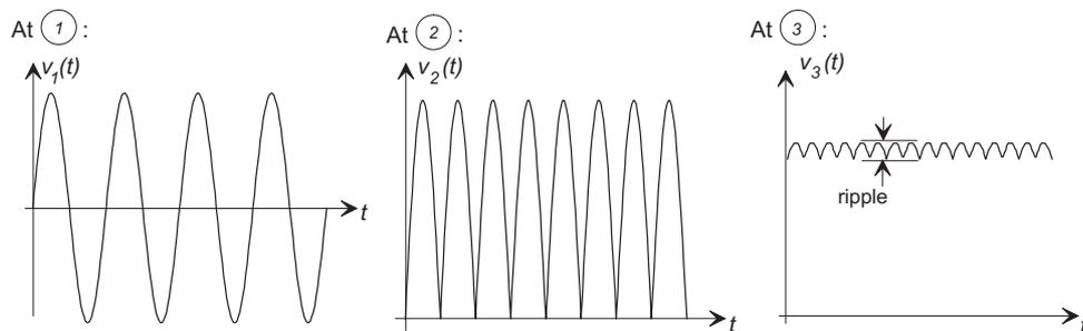
The filter acts to “smooth” the full-wave rectified waveform at **(2)** to produce a dc output at **(3)** with a very much reduced “ripple”.
