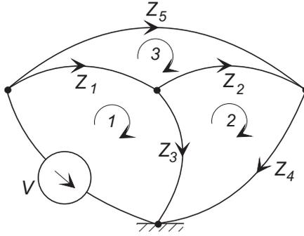
Define a set of (clockwise) loops as shown, ensuring that every graph branch is covered by at least one loop. The loops 1, 2 and 3 are somewhat arbitrary. We assume hypothetical continuous mesh currents  $i_1$ ,  $i_2$ , and  $i_3$  that flow around each loop.
