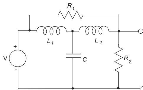
**Note:** This is a difficult example to solve using impedance reduction methods. It is, however, well suited to the mesh current method.
