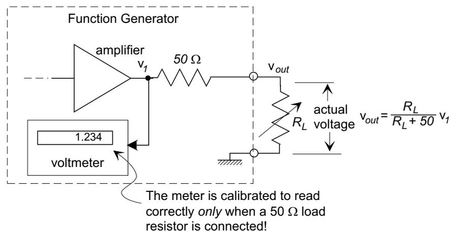
In the lab we have  $50\Omega$  terminator resistors connected across the output terminals so that the voltage reads correctly.
