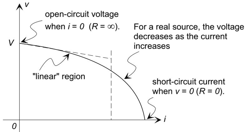
The voltage–current relationship is determined by the electrochemical reaction within the battery. It may be possible to define a region of operation at low currents in which there is an approximately linear relationship between voltage and current
