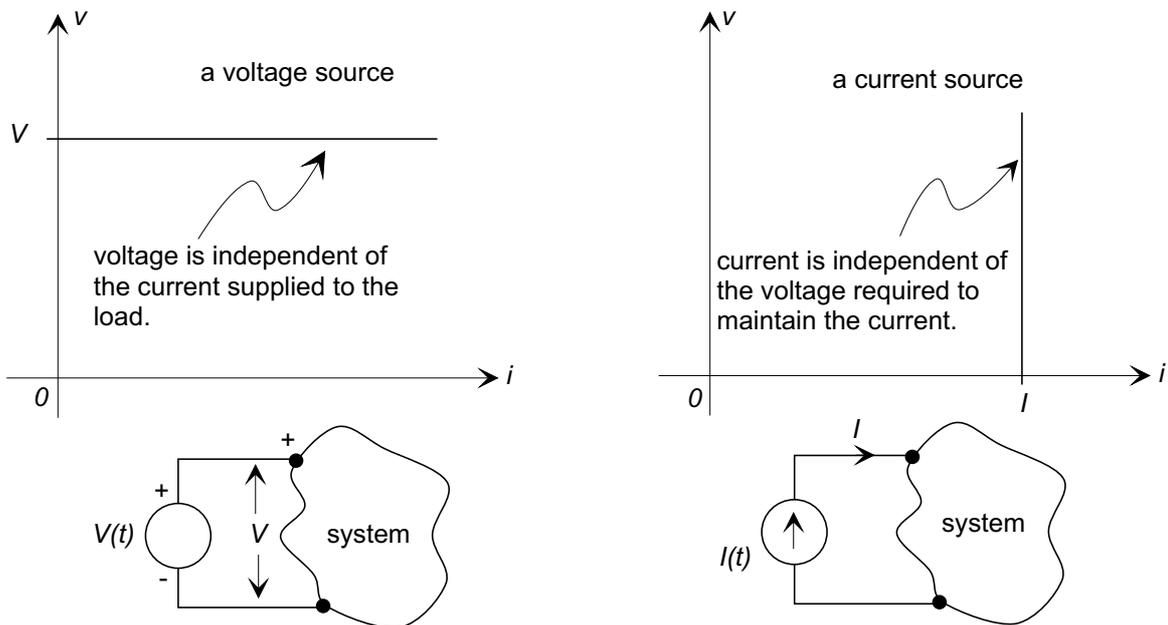
However, practical (real) sources do not have an ideal characteristic – they are power limited. For example we may think of a battery as an ideal voltage source - say with a 9 volt output, but if we were to measure the terminal voltage under increasing load currents
