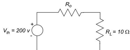
$$V_{th} = v_{oc} = 200 \text{ v.}$$
