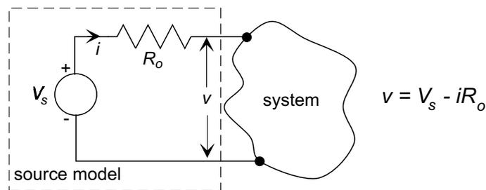
One way to do this is to model the real source(the battery) as an ideal voltage source  $V_s$  in series with a resistor  $R_o$  (the value of which is found experimentally). The voltage drop  $v_{R_o} = iR_o$  across the resistor accounts for the “droop” in the source characteristic.
